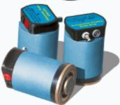
9265.070 CONNECTIONS Inner sensing ring: BNC int. / red 4mm socket Outer sensing ring: BNC ext. / black 4mm socket Shield / Guard: gray 4mm socket
