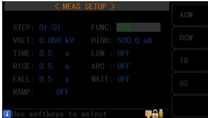
Figure 4.3.2 DC setup interface
