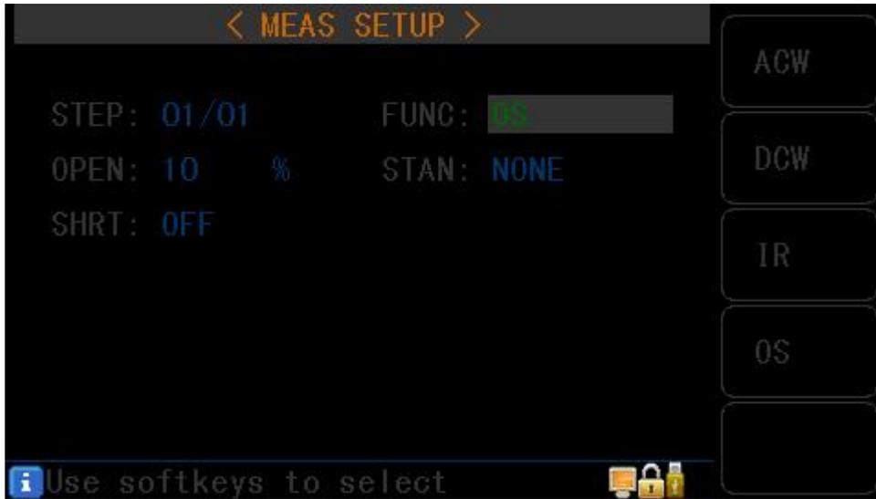
Figure 4.3.4 OS setup interface
