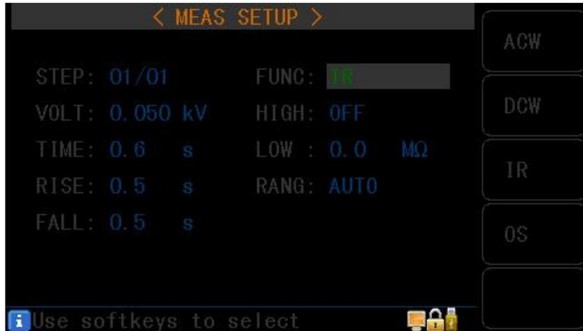
Figure 4.3.3 IR setup interface
