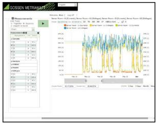
Load characteristics, current, voltage, power and much more can be displayed in separate or superimposed diagrams.
