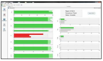
Evaluation of the measurement results in accordance with EN 50160 is possible in graphic as well as tabular format.
