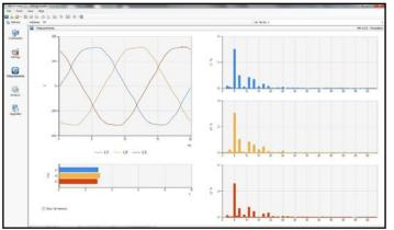
The real-time display indicates the system's harmonic load.
