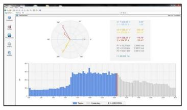
The vector diagram and the multimeter function (top half of the monitor) provide information regarding the momentary load status. The bar chart (bottom half of the monitor) indicates previous and anticipated daily load characteristics.
