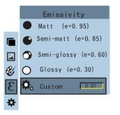
As shown in the figure, press " MENU/  $\oplus$  " key to enter the main menu and select "  $\epsilon$  "(emissivity) option and press "  $\blacktriangleright$  " key to enter the emissivity list.
