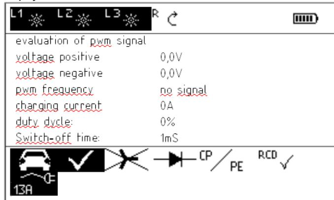
Display Multiple display with dot matrix, 240 x 128 pixels, diagonal: 10.7 cm (4.2")
